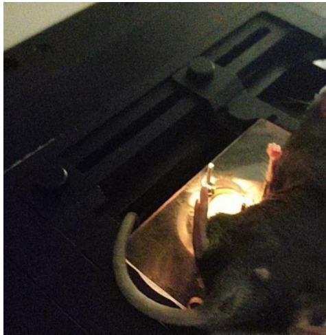
Figure 12: Fixation of the mouse on the microscope stage. A transparent resin window chamber holder whose size is equal to a microscope slide was installed.
